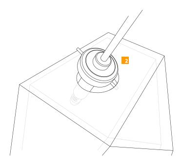
Once the fitter is inside of the top opening, rotate until the holding posts allow the lamp to sit center of the glass.
